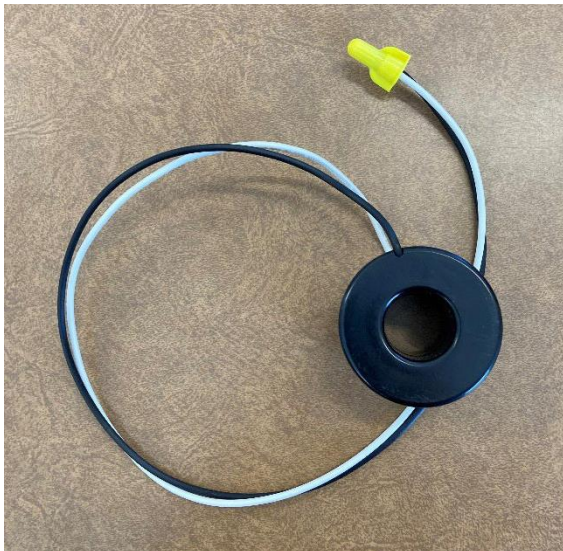
Current transformer – supplied by SCEC
