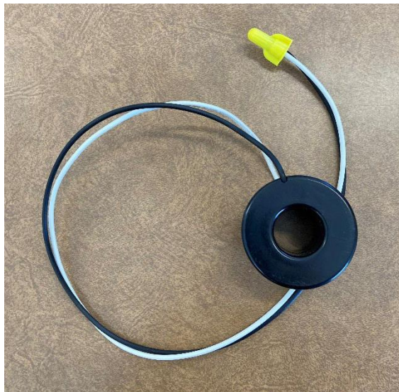
Current transformer – supplied by SCEC
